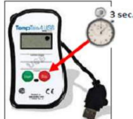
3. Press and hold the STOP button (1 to 3 seconds) until following icon appears
